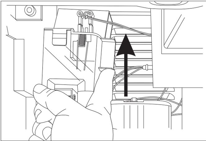
7. Locate drain plug and pull the drain plug out to drain the reservoir and evaporator. When draining is complete, return the plug to its original position.
