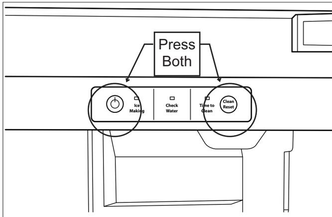
12. The auger motor alone will be operating for 10 minutes, after that the compressor will start and in about 5-8 minutes the machine will start to make ice. The Time to Clean light will now glow steady until the clean cycle is complete.
