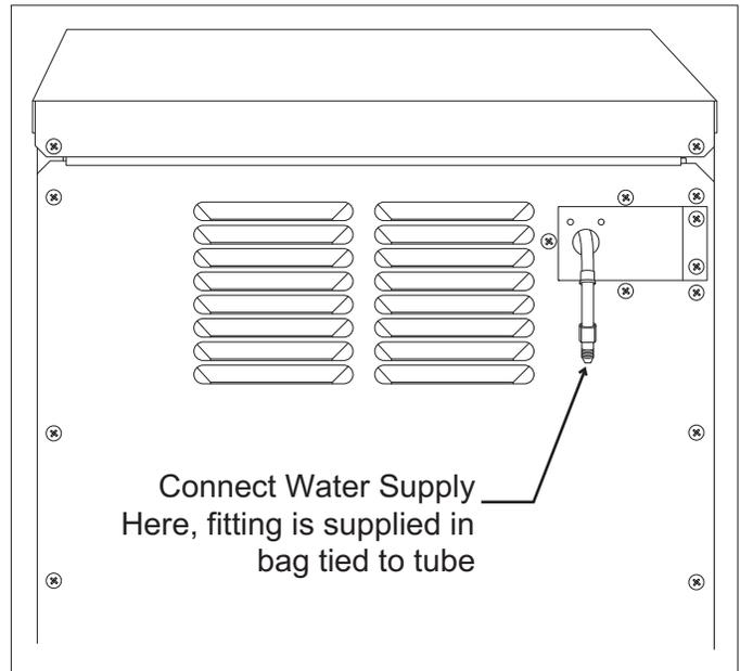
The water connection is at the back of the cabinet. Connect using a compression fitting, one is supplied tied to the water inlet tube at the back of the cabinet.
