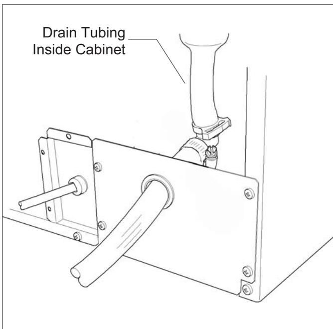
6. Cut an 8" piece of 5/8" ID X 7/8" OD tygon (clear plastic) tubing. Slide one end of the tube onto the outlet of the barbed connector and secure with a clamp. Leave the other end of the tube lying on the floor of the base pan until the unit is positioned over the floor drain.
