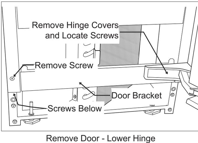
2. Slide hinges to the side and remove door from cabinet. Remove screws loosened in step 1 from both cross braces.
