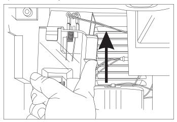
7. Locate drain plug and pull the drain plug out to drain the reservoir and evaporator. When draining is complete, return the plug to its original position.
