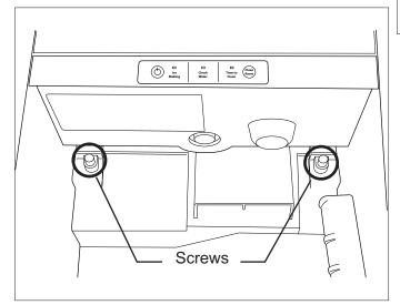
4. Remove the back panel of the bin by lowering it down past the scoop holder, feel free to rotate the scoop holder loop down to make more room.
