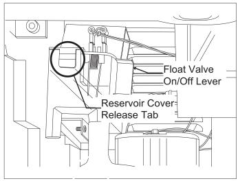
5. Push tab on front edge of reservoir cover and remove the cover. Note: Adjacent wires are low voltage and are not hazardous.
