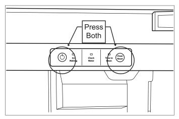
12. The auger motor alone will be operating for 10 minutes, after that the compressor will start and in about 5-8 minutes the machine will start to make ice. The Time to Clean light will now glow steady until the clean cycle is complete.
